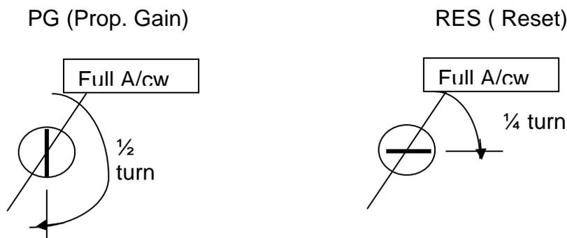
The RES adjustment controls the speed of response to a step change of output. Fully anti-c/w is the fastest and most likely to be unstable
